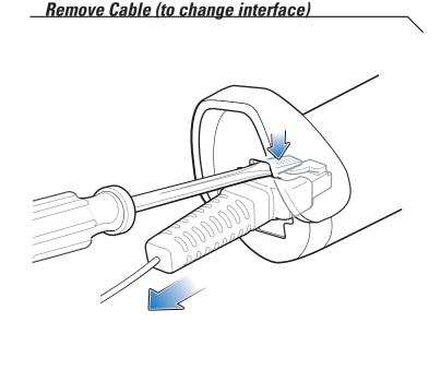
Note: An audible click sounds when the shielded cable is inserted correctly.
